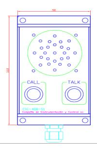
The substation CIC-408-S1, with call/ back button and 2W internal Loudspeaker, provides a talk-back speaker with CALL and TALK keys for privacy in the communications channel. The CALL key provides a call tone that sounds in the master station, and an intermittent green LED signals the line. The TALK key has to be pressed to transmit the audio from the substation through the speaker. Wall mounting.
